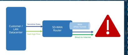
In this diagram we see Customer sensitive data being incorrectly steered direct to the Internet instead of going through the secure IPsec tunnel.
