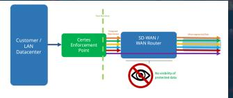
By adding a Certes Enforcement Point in-line we can mitigate the impact of this misconfiguration by protecting the sensitive data based on business risk before it gets to the SDWAN or WAN edge. This means that even if an SDWAN policy is incorrectly defined to send sensitive data "direct to net" there will be no business impact as the data will be fully protected and not visible to anyone other than the intended recipient.
